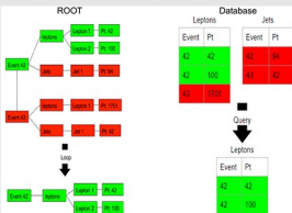
Figure 2. The figure on the left shows how data analysis is done in ROOT. The data is stored in a tree which contains all of the events and their objects. To identify interesting events, a loop is constructed in C++ to run over the events and objects. Leptons and jets are examples of the objects. The figure on the right shows how data analysis is done in the database. All of the objects are stored in tables and SQL queries are run against the tables to find interesting events.
